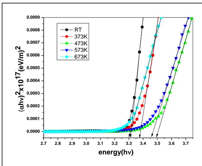
Fig.4. Plot of  $(\alpha hv)^2$  versus  $hv$  for the ZnO films at different substrate temperatures.
