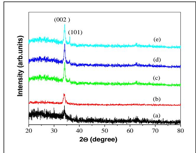
Fig. 2. X-ray diffraction patterns of ZnO thin films deposited at different substrate temperatures. (a) RT (b) 373K (c) 473K (d) 573K (e) 673K.
