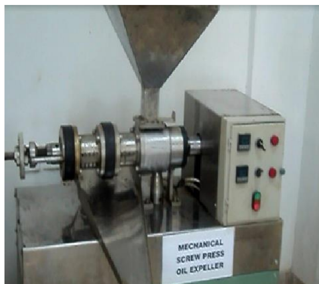
Figure 2. Extraction of Crude Oil through Mechanical Screw Oil Expeller
