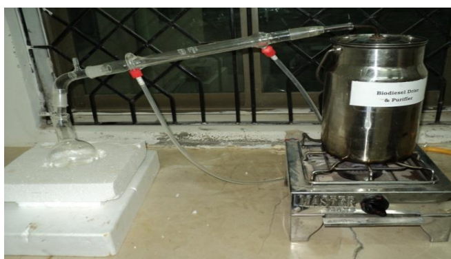
Figure 4: Drying of biodiesel & recovering of methanol through distillation process
