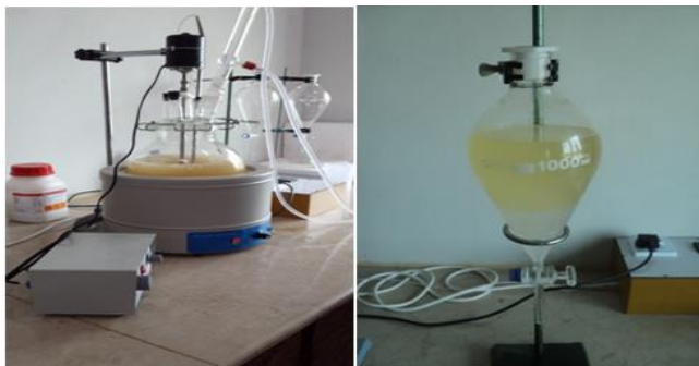
Figure 3: Production of Castor Biodiesel through Transesterification process
