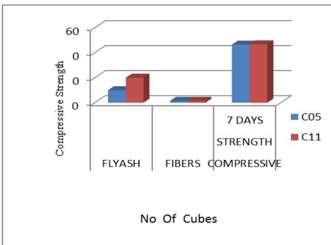
when, 10% & 20% of fly ash is added with 1.5% of fibers the compressive strength will be higher for the cube where 20% of fly ash along with 1.5% of fibers. Since, fly ash content is more.
