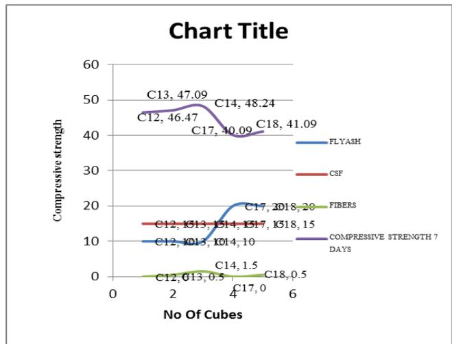
When 15% of Condensed Silica Fume(CSF) along with 0.5% & 1.5% of fibers are added to concrete cube the compressive strength increases when compared to fibers not added to CSF. But, if the fibre content increases more than 1.5% the self weight of concrete increases.
