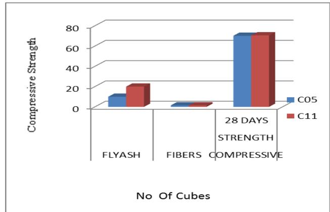
When 15% of Condensed Silica Fume(CSF) along with 10%, 20% fly ash and 0.5% ,1.5% of fibers are added to concrete cube the compressive strength increases when compared to fibers not added to CSF. But, if the fibre content increases more than 1.5% the self weight of concrete increases.
