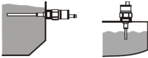
Figure 4 : Gasoline Level sensor
