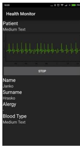
**Fig. 1** Screenshot of the application with displayed ECG data received from connected Raspberry Pi device.
