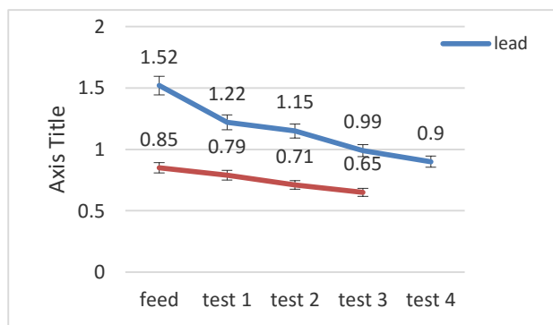
Figure 7.0 lead and arsenic concentrations after Lead decreased from 1.52% ( ) to 0.90% while arsenic decreased from 0.85% (concentrate without depressant) to 0.65%.
