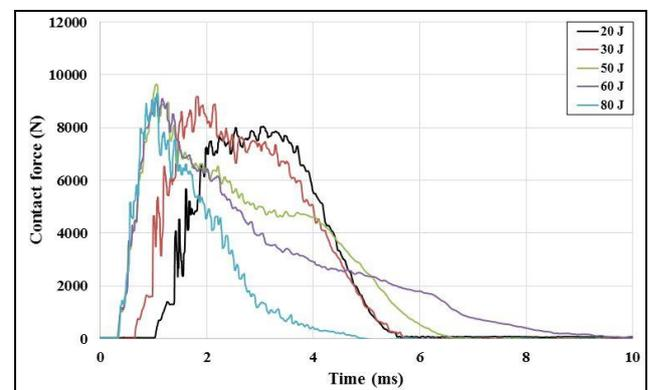
Figure 4: contact force-time diagram of glass fiber reinforced composites in different energy
