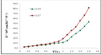
Figure (8): The specific detectivity (D\*)as a function of bias voltage of TiO<sub>2</sub>:ZnO at concentrations (5%, 7%) at RT
