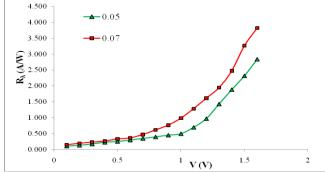
Figure (5): The responsivity as a function of bias voltage of TiO<sub>2</sub>:ZnO at different concentrations at 500°C.
