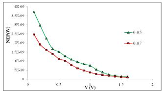
Figure (7): The noise equivalent power as a function of bias voltage of TiO<sub>2</sub>: ZnO at concentrations (5%, 7%) at 500°CC.
