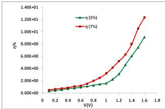
Figure (11): The quantum efficiency ( $\eta$ ) as a function of bias voltage of TiO<sub>2</sub>:ZnO at concentrations (5%, 7%) at 500°C
