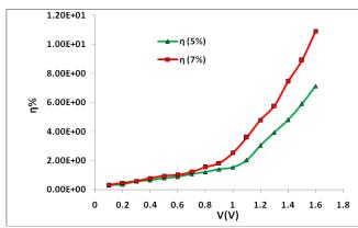
Figure (10): The quantum efficiency ( $\eta$ ) as a function of bias voltage of TiO<sub>2</sub>:ZnO at concentrations (5%, 7%) at RT.
