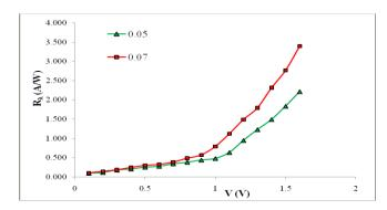
Figure (4): The responsivity as a function of bias voltage of TiO<sub>2</sub>: ZnO at different concentrations at RT.
