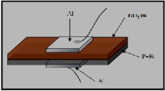
Fig.(1): Schematic device structure of the Al/TiO<sub>2</sub>: ZnO /PSi/Al heterojunction ultraviolet photodetector.
