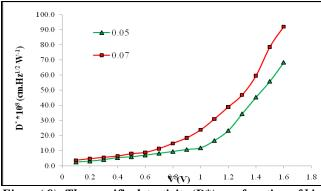
Figure (9): The specific detectivity (D\*) as a function of bias voltage of TiO<sub>2</sub>: ZnO at concentrations (5%, 7%) at 500°C
