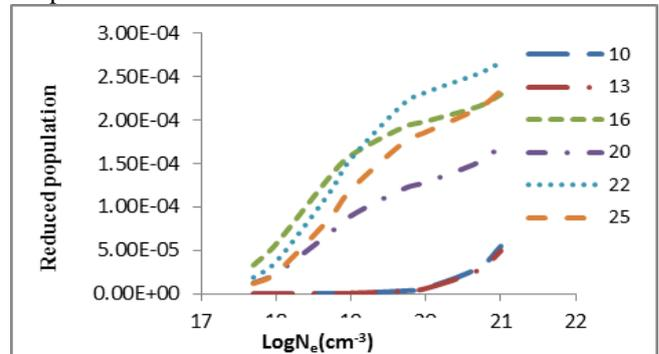
Fig.4 reduced population of  $Se^{34+}$  levels after electron collisional pumping as a function of the electron density at temperature 2000 eV
