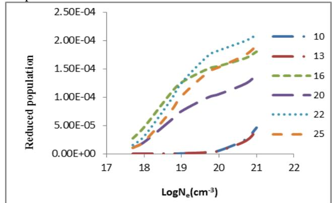
Fig.3 reduced population of  $Se^{34+}$  levels after electron collisional pumping as a function of the electron density at temperature 1500 eV
