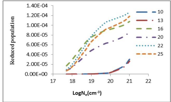
Fig.2 reduced population of  $Se^{34+}$  levels after electron collisional pumping as a function of the electron density at temperature 1000 eV
