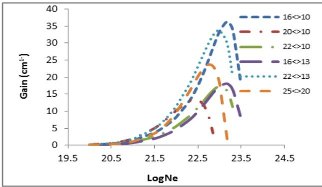
Fig.10 gain coefficient of possible laser transition against electron density at temperature 2500eV in Se<sup>34+</sup>
