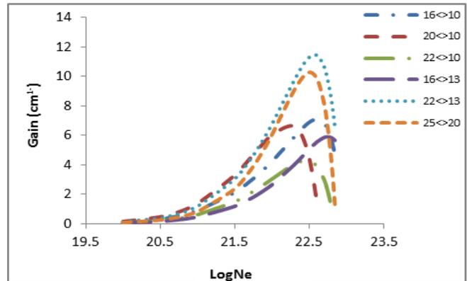
**Fig.7** gain coefficient of possible laser transition against electron density at temperature 1000eV in Se<sup>34+</sup>
