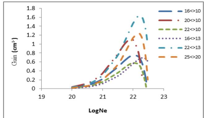
**Fig.6** gain coefficient of possible laser transition against electron density at temperature 500eV in Se<sup>34+</sup>
