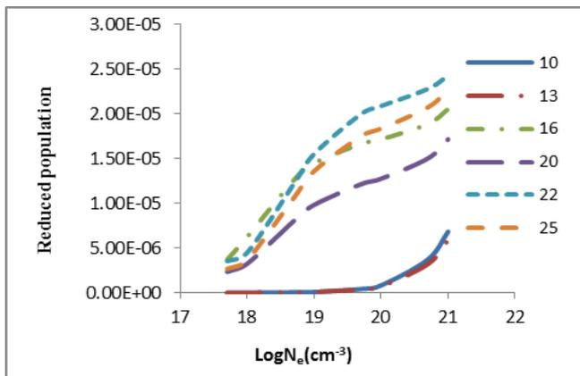
Fig.1 reduced population of  $Se^{34+}$  levels after electron collisional pumping as a function of the electron density at temperature 500 eV
