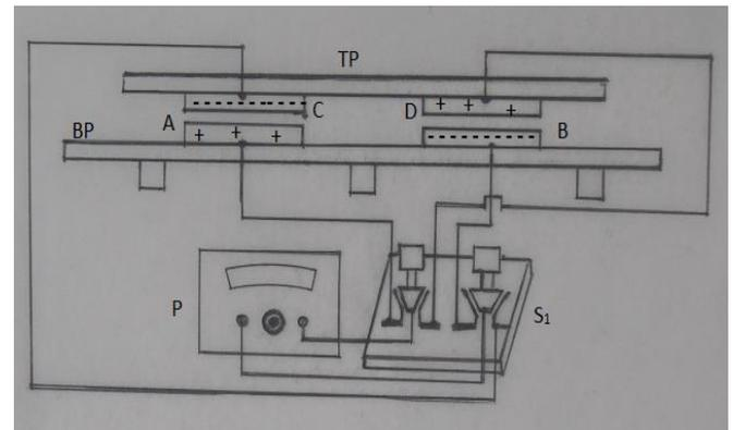
**Figure 3a.** Schematic diagram of the process employed for charging the metal plates through electrostatic induction. P- Variable voltage power supply, S<sub>1</sub>- Manually operated electrical switch, BP-Base plate (Bakelite), TP-Top plate (Bakelite), A,B,C,D- identical aluminium plates fixed symmetrically on Bakelite plates.
