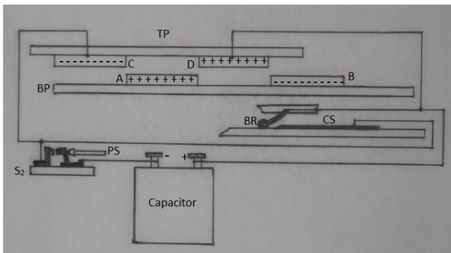
**Figure 3b.** Schematic diagram of the process employed for charging the capacitor due to the discharging current of the charged plates through it. BP-Base plate (Bakelite), TP-Top plate (Bakelite), A,B,C,D- identical aluminium plates fixed
