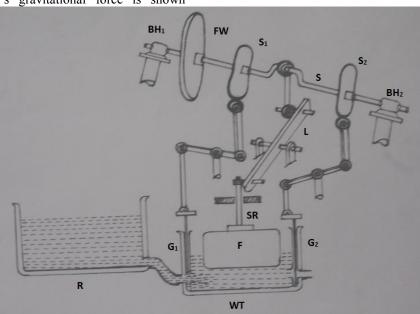
**Figure 2.** Schematic diagram of the contraption which makes use of the buoyant forces for energy generation. R-reservoir, WT-working tank, F-float,  $G_1$ -water inlet gate,  $G_2$ -water outlet gate, SR-stem rod, L-lever, S-shaft,  $S_1$  and  $S_2$  are mechanically operated gating system for  $G_1$  and  $G_2$ , respectively, FW-flywheel,  $BH_1$  and  $BH_2$ -ball bearing housings.
