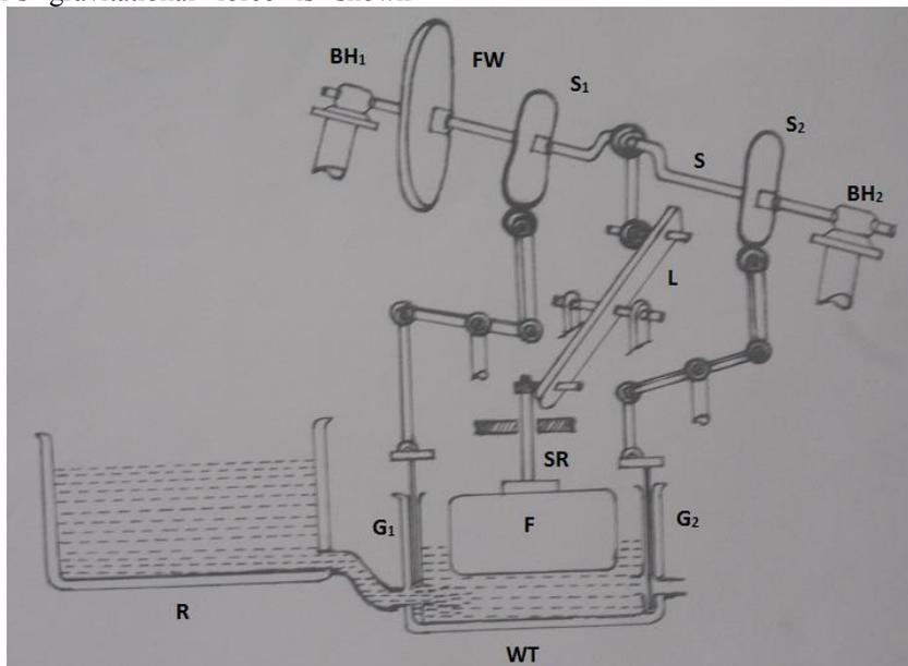
**Figure 2.** Schematic diagram of the contraption which makes use of the buoyant forces for energy generation. R-reservoir, WT-working tank, F-float, G<sub>1</sub>-water inlet gate, G<sub>2</sub>-water outlet gate, SR-stem rod, L-lever, S-shaft, S<sub>1</sub> and S<sub>2</sub> are mechanically operated gating system for G<sub>1</sub> and G<sub>2</sub>, respectively, FW-flywheel, BH<sub>1</sub> and BH<sub>2</sub>-ball bearing housings.
