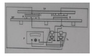
**Figure 3a.** Schematic diagram of the process employed for charging the metal plates through electrostatic induction. P-Variable voltage power supply, S<sub>1</sub>- Manually operated electrical switch, BP-Base plate (Bakelite), TP-Top plate (Bakelite), A,B,C,D- identical aluminium plates fixed symmetrically on Bakelite plates.
