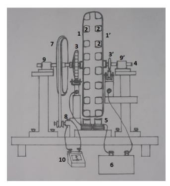
**Figure 1.** Schematic diagram showing the important components of the device for extracting energy from the permanent magnets. 1-1'-Bakelite discs, 2-polepieces of the permanent magnets, 3-3'-Switching system, 4-shaft, 5-electromagnet, 6-Battery (24 V), 7- pulley, 8- dynamo, 9-ballbearing housing, 10-ammeter.
