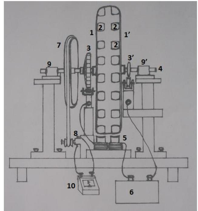
**Figure 1.** Schematic diagram showing the important components of the device for extracting energy from the permanent magnets. 1-1'-Bakelite discs, 2-polepieces of the permanent magnets, 3-3'-Switching system, 4-shaft, 5-electromagnet, 6-Battery (24 V), 7- pulley, 8- dynamo, 9- ballbearing housing, 10-ammeter.
