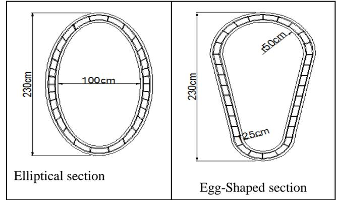
Fig.(5): Dimensions of the tested specimens
