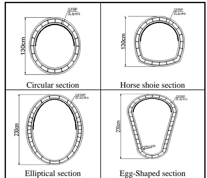
Fig.(6): Strengthened specimens
