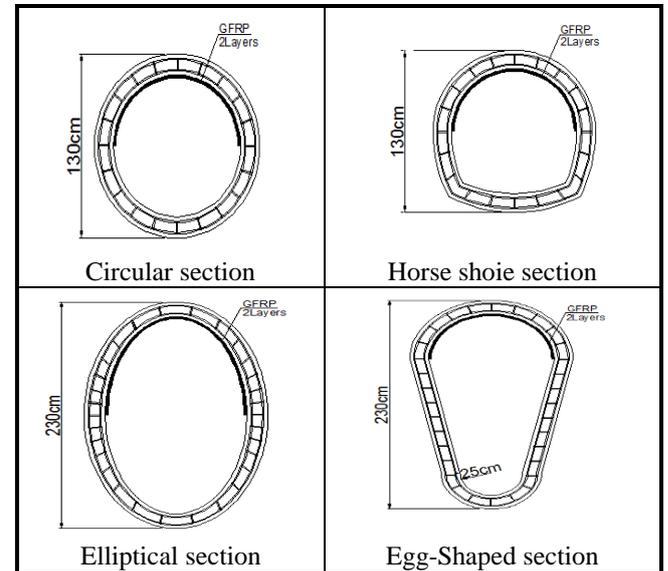
Fig.(6): Strengthened specimens
