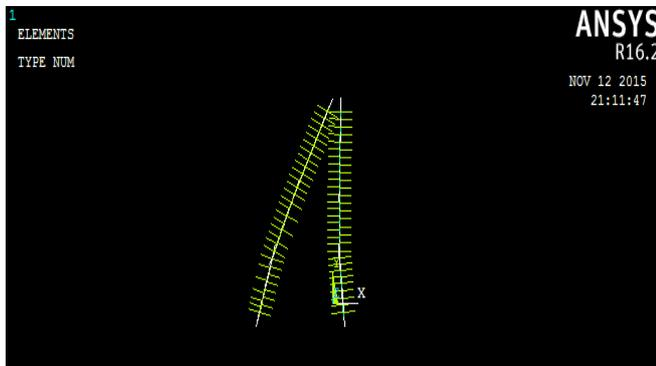
Fig. 3. Contact Elements between core-shell interfaces
