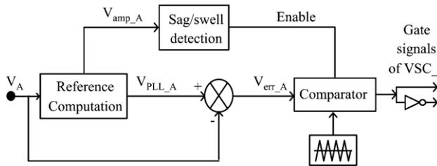
Fig. 2. Control block diagram of the series converter.
