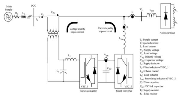
Fig. 1. Schematic diagram of UPQC.
