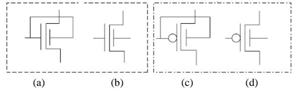
Fig 10: Schematic symbols of a) SG nFinFET b)IG nFinFET c) SG pFinFET d) IG pFinFET
