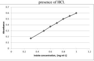
Fig. 8: Calibration graph for indole and 2,4,6-trimethoxybenzaldehyde in the presence of HCl.
