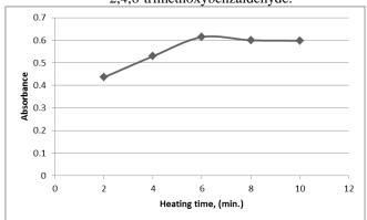
FigFig. 7: Effect of heating time on the reaction of 1 µg ml<sup>-1</sup> indole and 2,4,6-trimethoxybenzaldehyde in the
