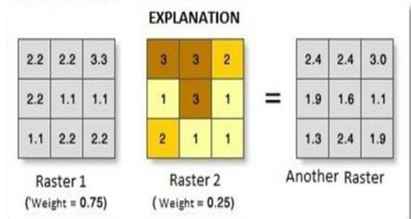
Fig 2. Tool Operating weighted sum, Source: Manual of Software Arcgis 10.1
