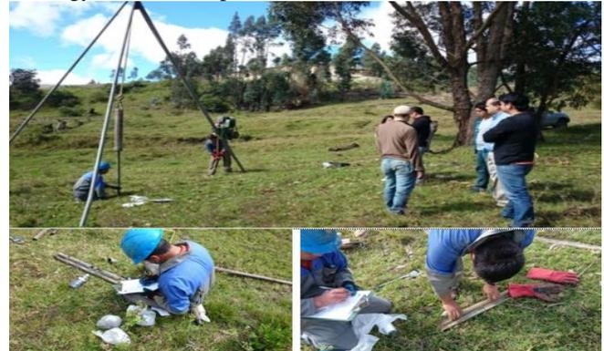
Fig 4. Obtaining samples of the Shelby tube in the pilot area.
