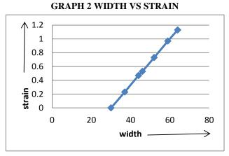
Fig.5 Width VS Strain From Fig.5, the width of aluminium sheet increases the strain values of aluminium sheet also increases gradually.
