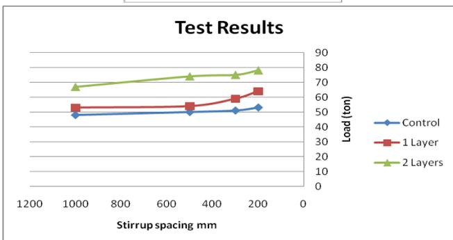
Fig.(6): comparison between tested specimens in group G1
