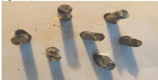
**Figure 11a: Types of fracture of strand 6**
