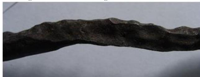
**Figure-7: Wear, corrosion & pittings in one wire**
