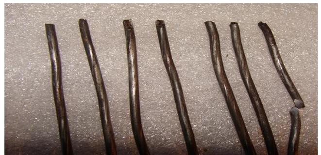
**Figure 10 (e-II): Types of fracture of Strand 5 with one wire broken from the middle**
