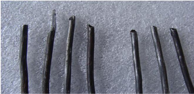
**Figure 11: Types of fracture of strand 6**
