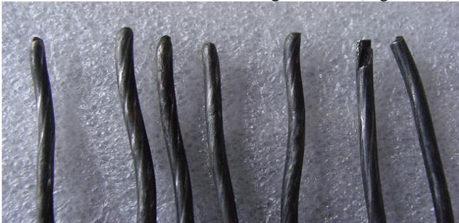
**Figure 10b: Types of fracture of strand 2**
