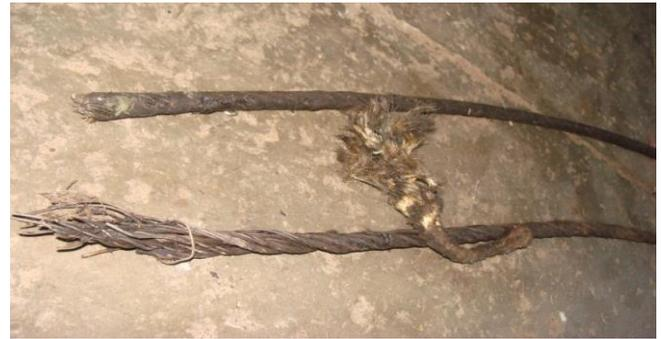
Figure 7: upper one – Fresh piece, Lower one - Broken end
