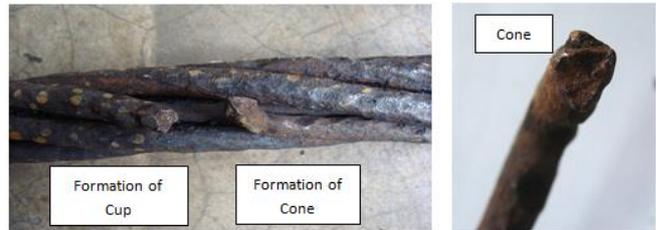
**Figure 6: After cleaning of failure broken end**
