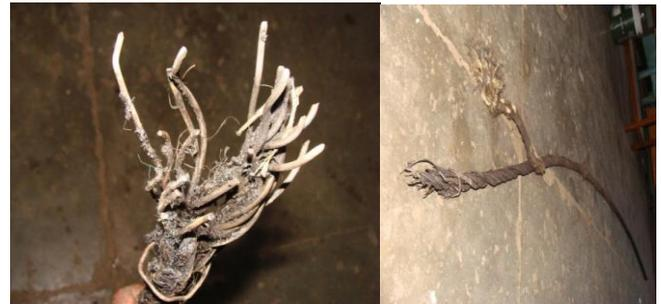
Figure 8: Fracture Rope Samples showing broken surfaces
