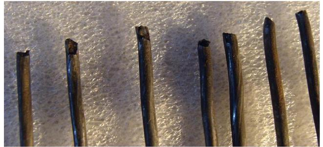
**Figure 10d: Types of fracture of strand 4**
