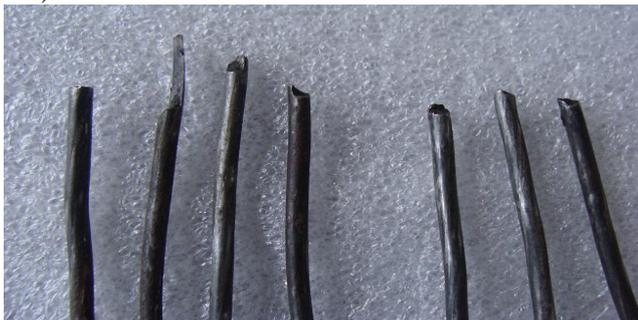
**Figure 10C: Types of fracture of strand 3**
