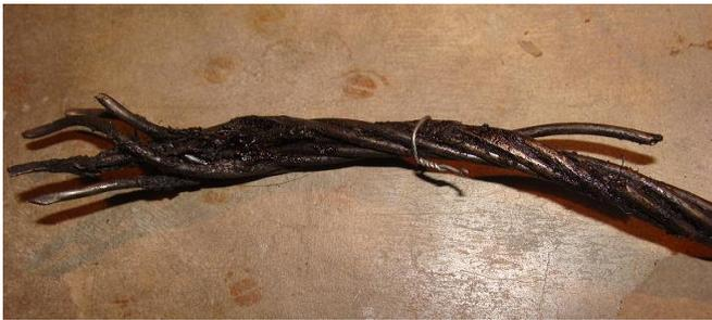
**Figure 10: Broken wire of strand 1**
