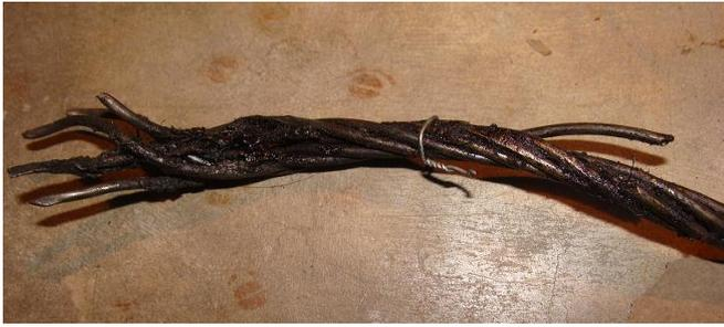
**Figure 10: Broken wire of strand 1**
