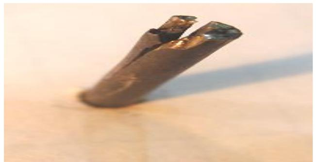
**Figure 10(e-III): Types of fracture of Strand 5**
