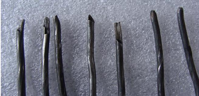
**Figure 10a: Types of fracture of strand 1**
