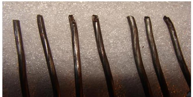
**Figure 10(e-I): Types of fracture of strand 5**
