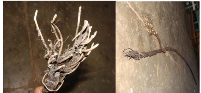
Figure 8: Fracture Rope Samples showing broken surfaces
