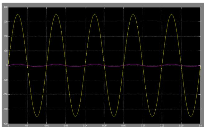
Fig 11 inverter voltage and current
