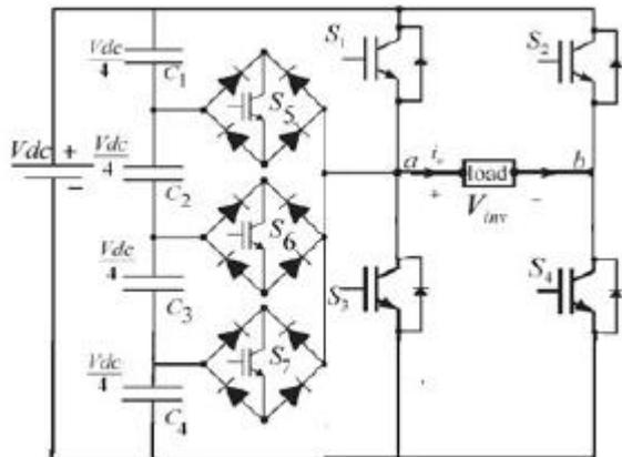
Fig. 9. Nine-level inverter for switching operation.
