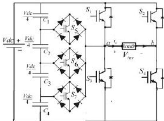
Fig. 9. Nine-level inverter for switching operation.
