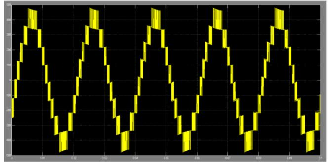
Fig 13 inverter output voltage
