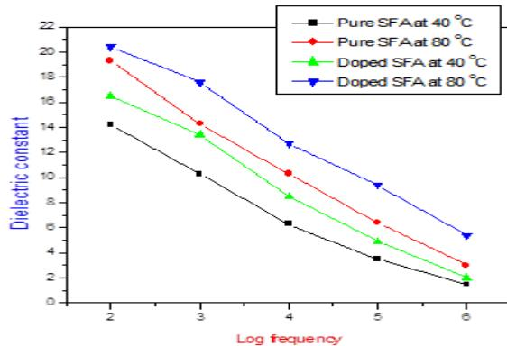
Fig.3: Variation of dielectric constant with frequency for pure and nickel chloride doped sodium fluoro antimonite (SFA) crystals
