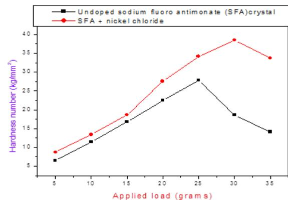
Fig.5: Variation of hardness number with applied load for nickel chloride doped sodium fluoro antimonate ( $\text{Na}_3\text{Sb}_4\text{F}_{15}$ ) crystals
