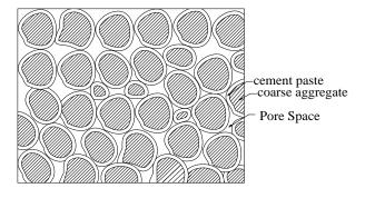
Figure 1 The schematic model of pervious concrete
