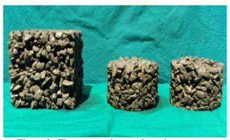
Figure 2 The cast specimens of pervious concrete
