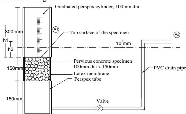
**Figure 3 Falling head permeability test setup**
