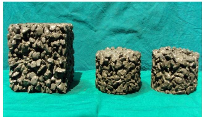
**Figure 2 The cast specimens of pervious concrete**
