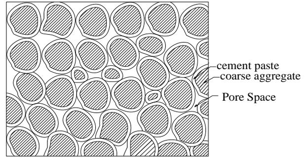
**Figure 1 The schematic model of pervious concrete**
