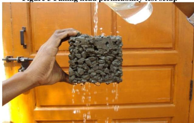
**Figure 4 Percolation of water through pervious concrete**
