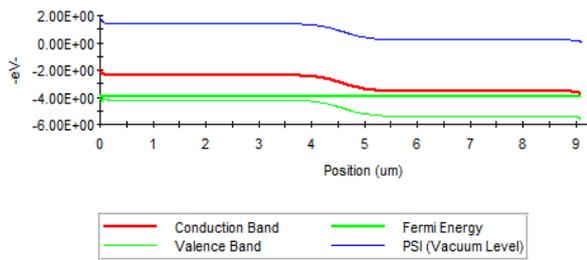
Fig. 4 Band-diagram of our proposed solar cell model
