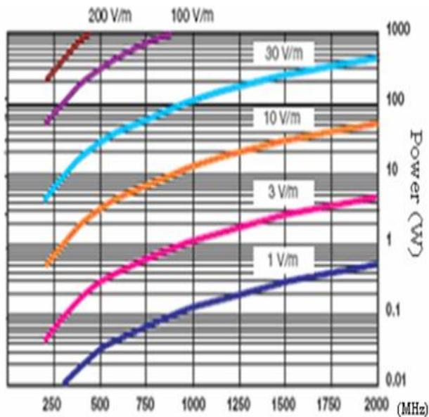
Fig. 4: Power Required for a Given Field Strength for IEC 61000-4-20
