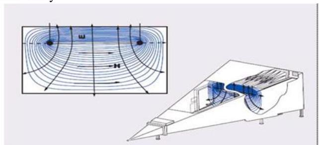
Fig. 2: EM Field Distribution in the GTEM Cell
