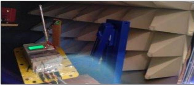
Fig. 6: DUT fixed on manipulator inside GTEM
