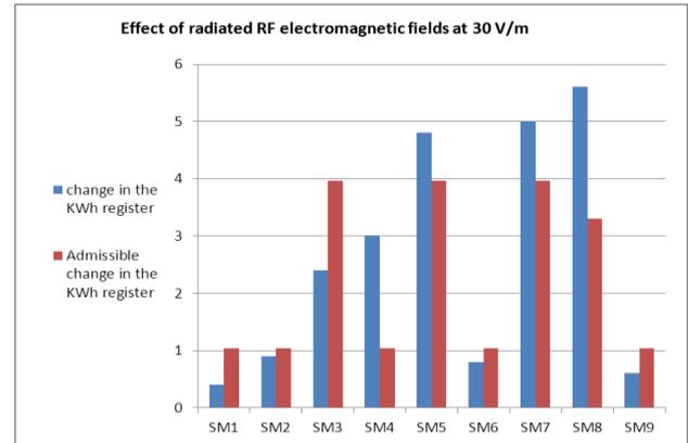
Fig. 7: Effect of radiated RF electromagnetic fields at 30 V/m
