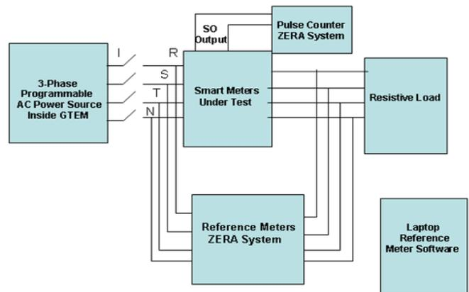
Fig. 5: Setup for testing three-phase watt-hour meters
