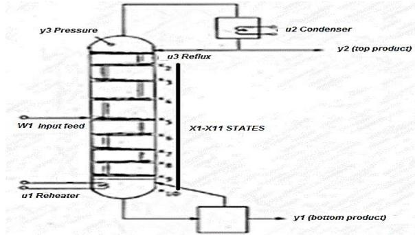
Fig. 2 Binary distillation column with pressure variation
