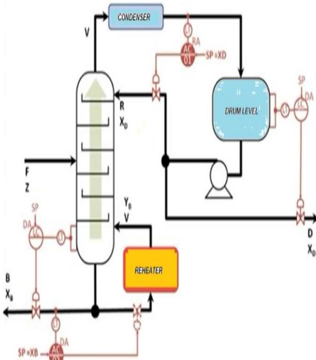
Fig. 7 Control scheme in where shown the sensors and actuators that must handle with the Fuzzy controller for output values desired. Photo Source: <http://www.youtube.com/watch?v=sYIkyDQVTzA&list=PL995A30D46244C35B>
