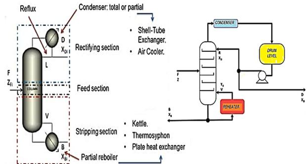
Fig. 1 In the left figure the stages shown operating of a binary distillation tower and in the right of this figure a distillation tower with a drum to control the level of reflux. Source photograph: left <http://www.youtube.com/watch?v=jcCZAUKfLKc>, right <http://www.youtube.com/watch?v=sYIkYDQVTzA&list=PL995A30D46244C35B>
