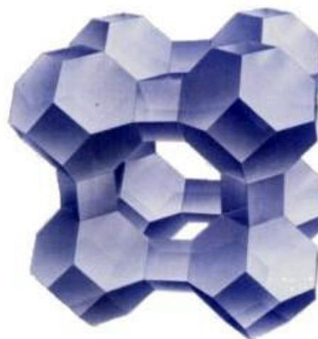
Figure 4. Molecular Sieve Type A
