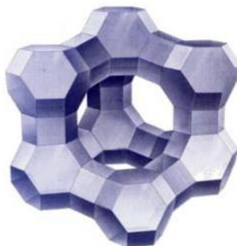
Figure 5. Molecular sieve type-X
