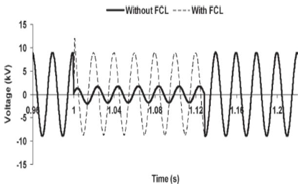
Fig. 9. PCC voltage of the A phase without and with the proposed FCL.
