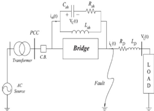
Fig. 3. Single-line diagram of the power system.
