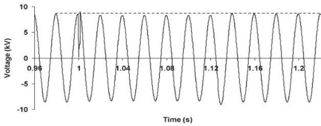
Fig. 11. PCC voltage of the A phase during the fault in the nonideal case
