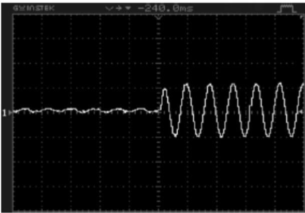
Fig. 16. Capacitor voltage during fault (voltage/div.: 50 V;
