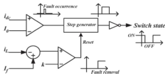
Fig. 2. Control circuit of the proposed FCL
