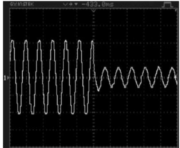
Fig. 14. PCC voltage without using the FCL (voltage/div.: 50 V; time/div.:25 ms).
