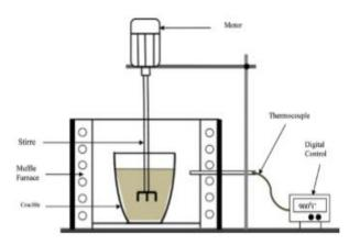
Figure 2. Schematic view of setup for stir casting (color figure available online).
