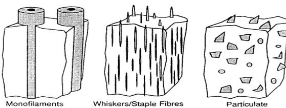
**Figure 1.** Schematic presentation of various types of metal matrix composites [4].
