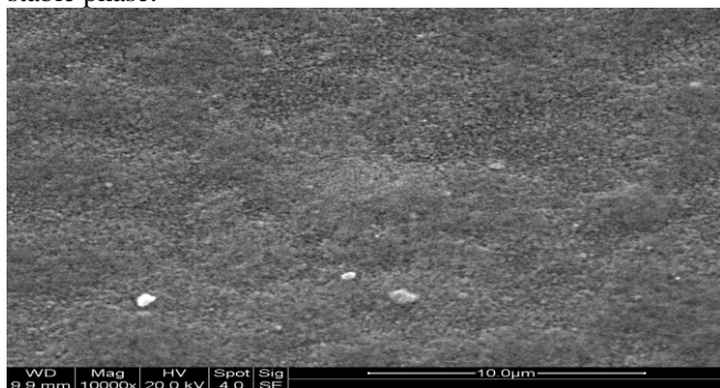
Figure 3. SEM image of TiO 2 thin film
