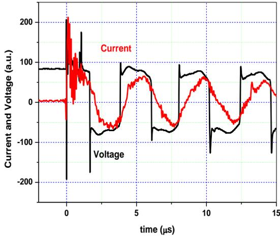
Figure (2): Current-voltage characteristics of pulsed plasma jet
