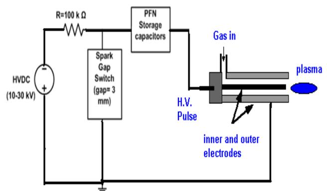
Figure (1): A schematic of the APPJ discharge
