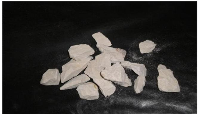
Feldspar is the most important group of rocks forming silicate (tectosilicate) minerals. The acid intrusive rocks (pegmatite) are the chief source of Feldspars.
