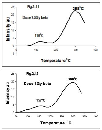
Fig. 2.11 shows the glow curve of as received Feldspar sample irradiated with beta dose of 2.5Gy by  $Sr^{90}$ .Here glow curve exhibits one broad peak at temperature  $116^{0}C$  and intensity 2.79au and one well resolved peak at temperature  $298^{0}C$ .,with intensity of 22.55au.
