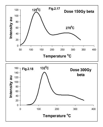
Fig. 2.17 shows the glow curve of as received Feldspar sample irradiated with beta dose of 150Gy by  $Sr^{90}$ .Here glow curve exhibits one well resolved peak at temperature  $125^{0}C$  and intensity 111.73 and one well resolved broad peak at
