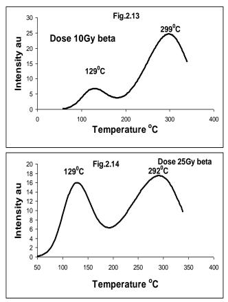
Fig. 2.13 shows the glow curve of as received Feldspar sample irradiated with beta dose of 10Gy by  $\mathrm{Sr}^{90}$ .Here glow curve exhibits one broad peak at temperature129<sup>o</sup>C and intensity 6.72au and one well resolved peak at temperature 299<sup>o</sup>C., with intensity of 24.57au.here the intensity of both the peaks are increased.
