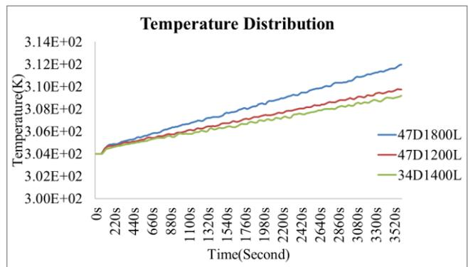
Fig.14. Temperature development for different geometries with 45° inclination
