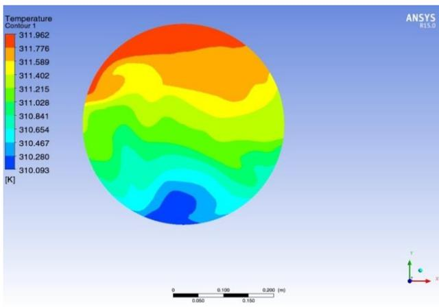
Fig.10. Temperature Stratification in the tank for 45° inclination
