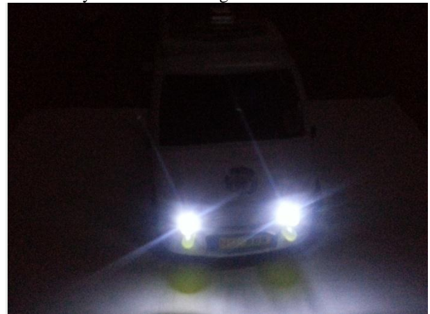
Fig 7: Vehicle in the dark with High Beam lights on and Low Beam off.
