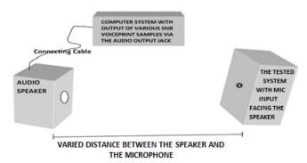
Fig. 3: Voice Recognition Experimental Setup
