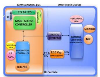
Fig. 2: System Architecture of the Developed System
