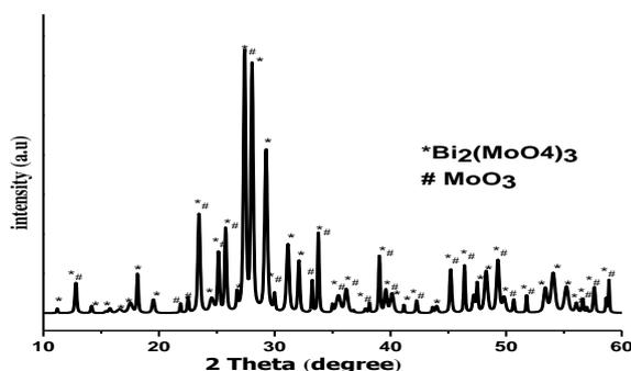
Fig 1. XRD pattern of resulting powder obtained from Bismuth nitrate, Molybdenum oxide and Glycine in water, heat treated at  $400^\circ\text{C}$  for 4 hr.
