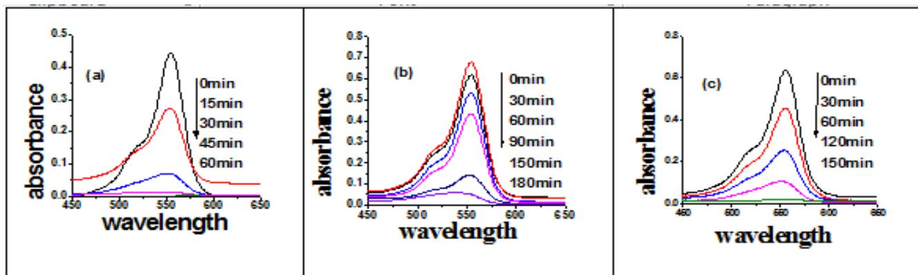
Fig. 4. Temporal evolution of spectral changes of Rh-B aqueous solution as a function of irradiation time in presence of (a) photocatalyst +  $\text{H}_2\text{O}_2$ , (b) photocatalyst +  $\text{H}_2\text{O}_2$  +  $\text{HCO}_3^-$ , and (c) photocatalyst +  $\text{H}_2\text{O}_2$  + manitol
