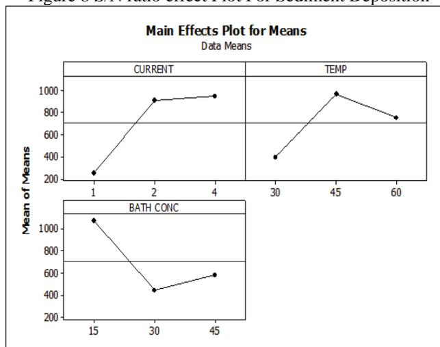
Figure 9 mean effect Plot For conventional Deposition
