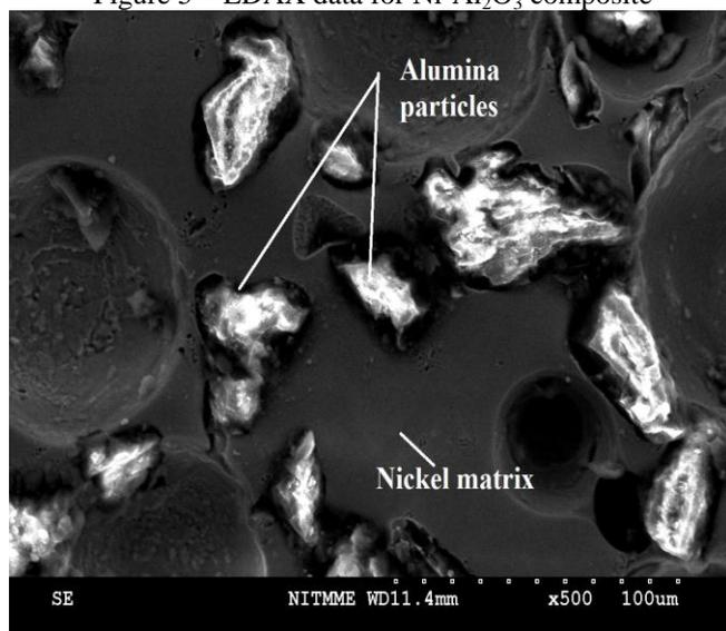
Figure 6 SEM micrographs of Ni- Al<sub>2</sub>O<sub>3</sub> composite coating
