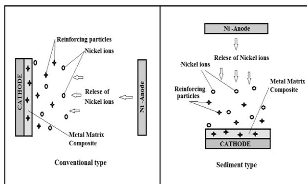
Figure 3 Conventional type and sediment type electro-deposition
