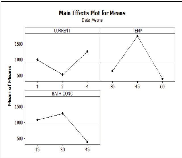
Figure 9 mean effect Plot for Sediment Deposition
