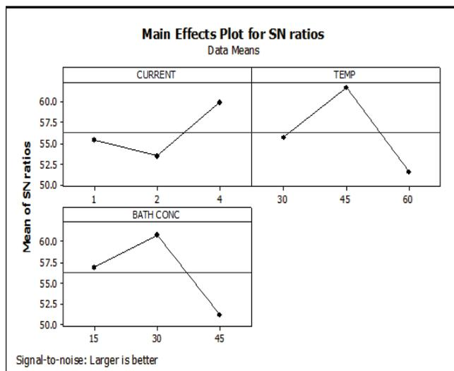
Figure 8 S/N ratio effect Plot For Sediment Deposition
