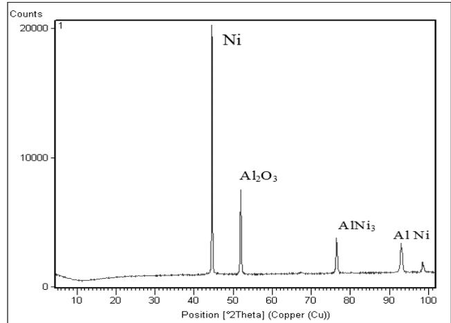
Figure 4 – XRD pattern of Ni-Al<sub>2</sub>O<sub>3</sub> composite
