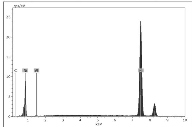
Figure 5 – EDAX data for Ni-Al<sub>2</sub>O<sub>3</sub> composite
