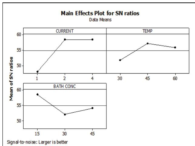
Figure 7 S/N ratio effect Plot For conventional Deposition
