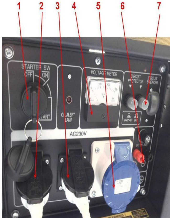
Figure 1: Command-control-protection panel and output power generator.
