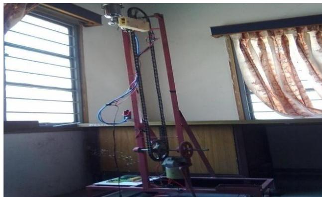
Figure 2: Intelligent Automatic Wall Painting Machine
