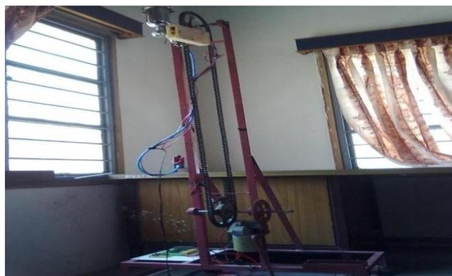
Figure 2: Intelligent Automatic Wall Painting Machine
