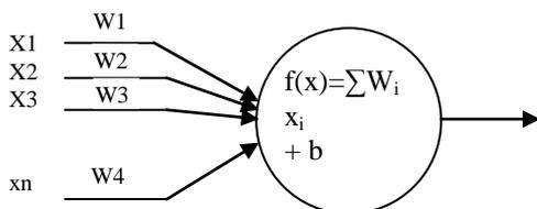
Figure 1: Theoretical Model of a Neuron
