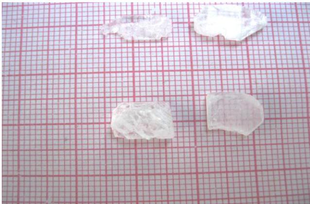
Fig. 1. Photograph of the grown  $\text{KSbF}_4$  crystal
