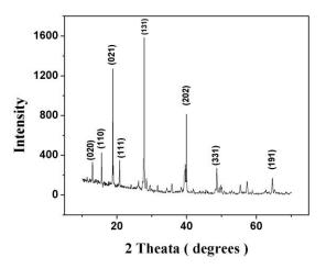
Fig. 4. Indexed observed XRD Pattern of K<sub>2</sub>SbF<sub>5</sub> crystal
