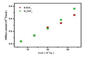
Fig. 8. Variation of stiffness constant with load for  $KSbF_4$  and  $K_2SbF_5$  crystals
