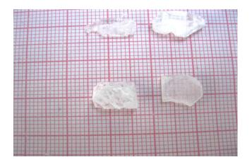
Fig. 1. Photograph of the grown KSbF<sub>4</sub> crystal
