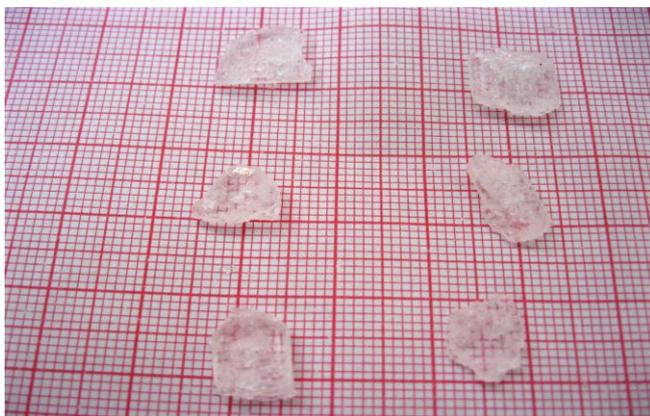
Fig. 2. Photograph of the grown  $\text{K}_2\text{SbF}_5$  crystal
