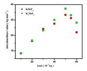
Fig. 5. Variation of microhardness with load for KSbF<sub>4</sub> and K<sub>2</sub>SbF<sub>5</sub> crystals.
