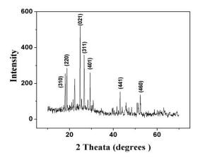
Fig. 3. Indexed observed XRD Pattern of KSbF<sub>4</sub> crystal
