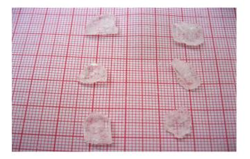
Fig. 2. Photograph of the grown K<sub>2</sub>SbF<sub>5</sub> crystal
