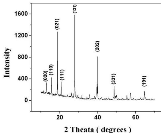
Fig. 4. Indexed observed XRD Pattern of  $\text{K}_2\text{SbF}_5$  crystal
