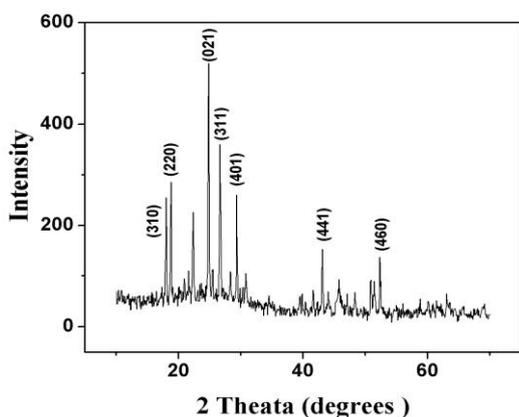
Fig. 3. Indexed observed XRD Pattern of  $\text{KSbF}_4$  crystal
