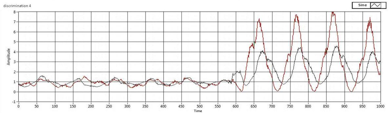
Figure 9(c), Forward and backward discriminated traveling waves in BB fault condition.
