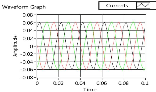
Figure 6(b), System 3 phase current signal during normal conditions.
