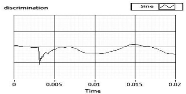
Figure 7(b), resultant discrimination signal during BB fault conditions.
