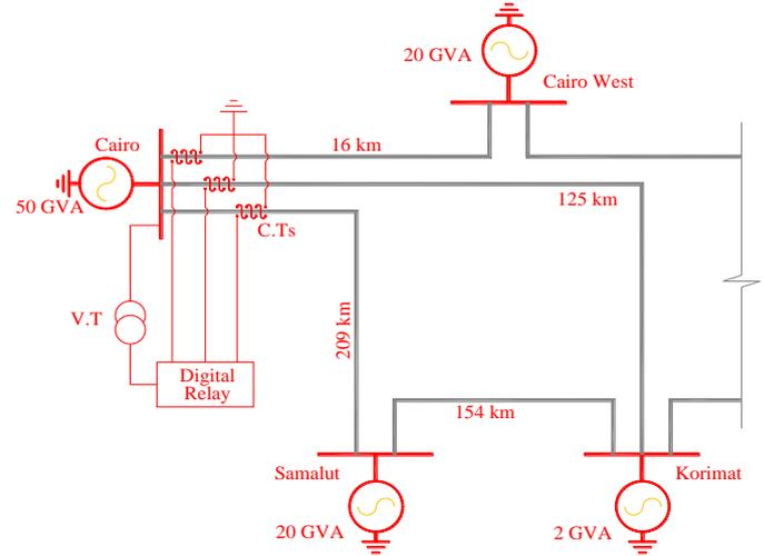
Figure 1. 500 kV, typical network used in simulation
