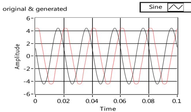
Figure 6(a). Input phase voltage and complementary generated signal during normal conditions.
