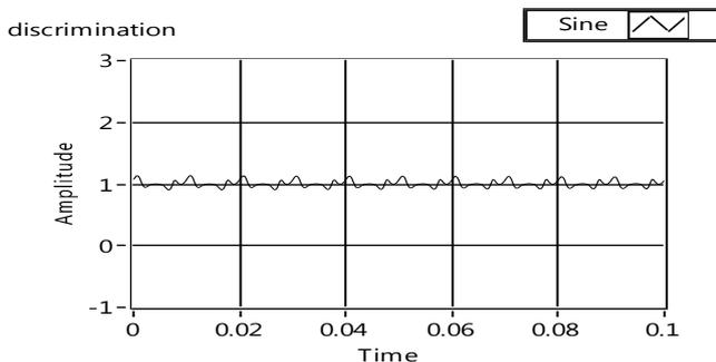
Figure 6(c), resultant discrimination signal during normal conditions.
