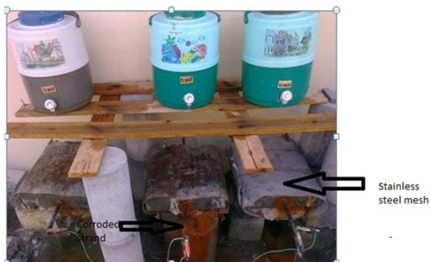
Fig. 1 Block Specimen subjected to 5% NaCl Solution
