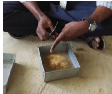
Fig. 2 Coir fibre cut into required size
