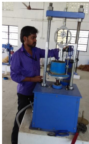
Fig. 4 Soaking of sample Fig. 5 CBR Test in loading frame
