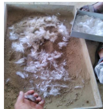
Fig. 3 Mixing of fiber and soil
