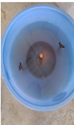
Fig. 4 Soaking of sample Fig. 5 CBR Test in loading frame
