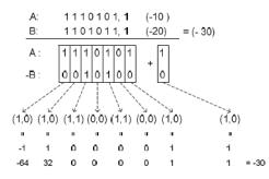
Fig. 4 RB encoding using one's complement airthematic
