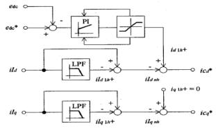
Fig. 4. DC voltage regulation circuit.
