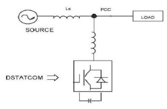
Fig. 1. Block diagram of DSTATCOM circuit.
