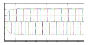
Fig.9. load current with D-STATCOM, x-axis in Time (sec), y-axis in amplitude (v)
