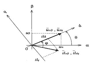
Fig. 2. Space vector representation voltage and current.
