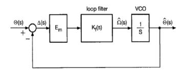
Fig. 3. Linearized model of three-phase PLL system.
