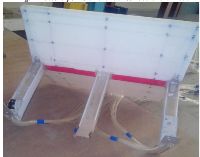
Fig.3 Perspex sheet model of Trough canopy roof
