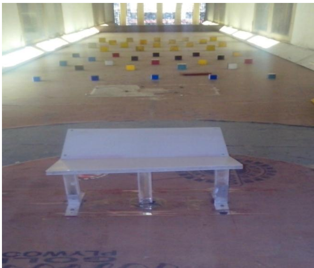
Fig.4 Trough canopy roof model inside wind tunnel
