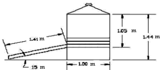
Fig. 2 Schematic diagram of Seasoning Chamber
