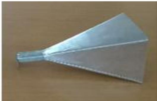
Figure-2 Fabricated horn antenna
