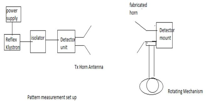
Figure-3 Radiation pattern setup
