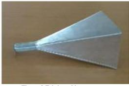
Figure-2 Fabricated horn antenna
