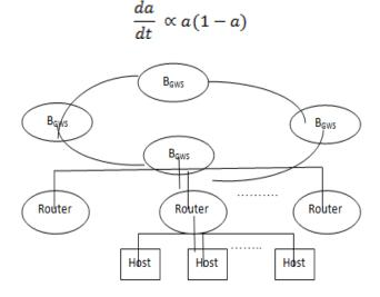
Figure 2.1: Hierarchical relationship among  $B_{GWS}$ , Routers and Hosts. Ordinary hosts are one level below routers which are one level below  $B_{GWS}$ .
