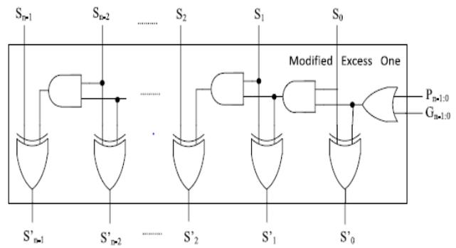
Fig. 5. Modified Excess one unit
