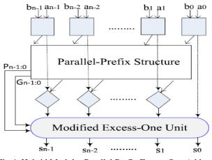
Fig.4. Hybrid Modular Parallel Prefix Excess One Adder
