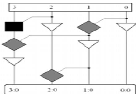
Fig. 3. 4 bit BK Adder Structure
