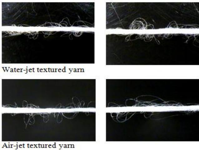
Figure 2. Water-jet and air-jet textured yarns
