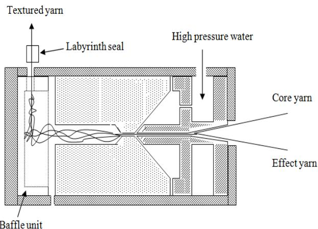
Figure 1. Schematic diagram of the water-jet texturing nozzle
