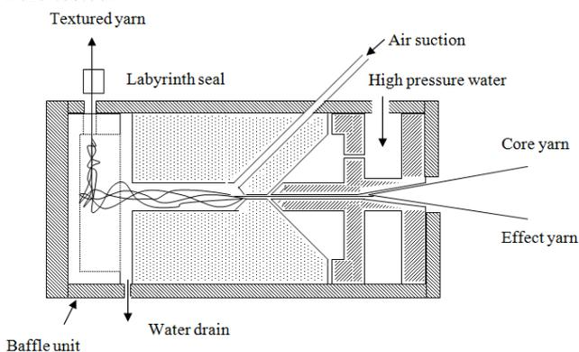
Figure 3. Schematic diagram of the Water/air-jet texturing nozzle.
